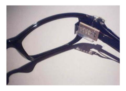
Wearable peripheral display (using tiny LEDs) embedded in a pair of eyeglasses delivers notification cues in a private, subtle and non-obtrusive way
